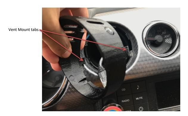
Center of the gauge, line mount up straight as possible in the orientation shown here. Mount can always be readjusted later to your liking.
