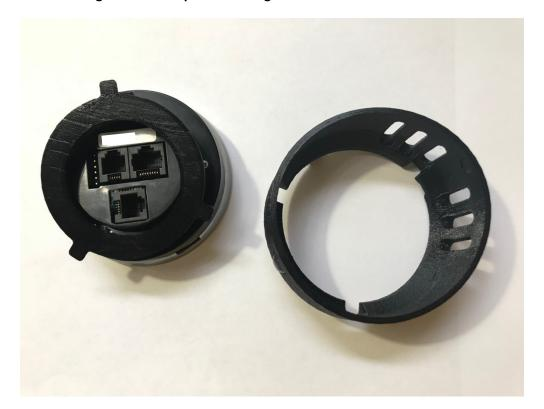
Step 3: Install the vent mount where the vent used to be. Squeeze the vent mount where the tabs are and push till mount locks in place.
