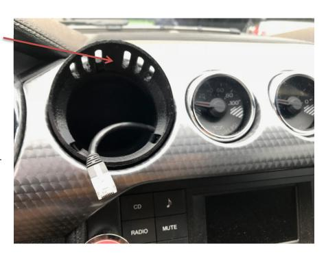
Step 4: Plug cable into nGauge before installing adapter into vent mount. Line up the three tabs on the adapter to the three slots on the vent mount. It can only slide in one correct way.
