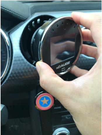
Step 5: Push in nGauge with adapter all the way in until the magnets engage, and that's it! Enjoy your new magnetic nGauge vent mount! Easily removable to get access to your micro sd card whenever you need to update or add a new tune.
